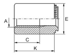
Female thread A = M3Height K = 11Min distance to edge = 4.0Outer diameter E = 7Plate thickness = 0.8 to 1.0
